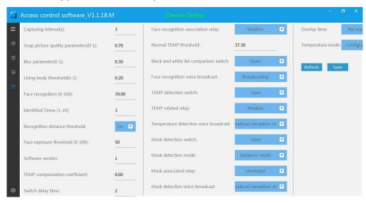
**Capturing interval:**Set the face capture interval to avoid repeated snapping of pictures in a short time.
